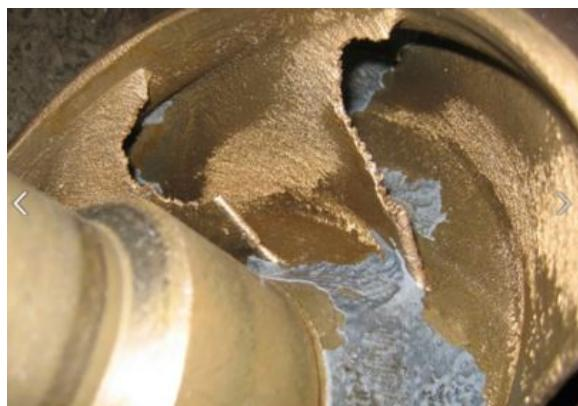
**Figure 2.** Uncontrolled cavitation can lead to damage of adjacent components or surfaces.
