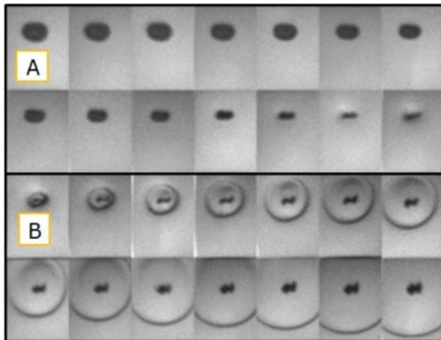
**Figure 1.** **A**, Collapse of the vapor cavity and **B**, formation and expansion of the shockwave.
