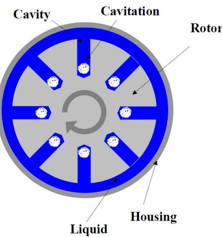
**Figure 3.** Specialized spinning rotor with cavities.
